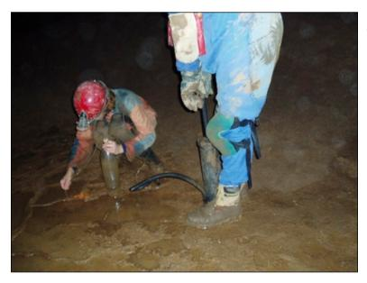
Figure 8.4: Apparatus for aspirating water in pools. After aspiration, the water is filtered. through a net or filtering bottle (Fig. 8.3) in order to recover the epikarst fauna (Photo: Daniel W. Fong).
