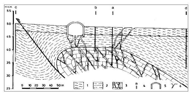
Figure 7.5: Hydrogeological profile of the Sv. Ivan spring (1 - Quaternary clays, 2 - flysch beds, 3 - karstified limestones, 4 - research borehole, 5 - collection reservoir, 6 - periodic spring) (Hidroprojekt-ing 2000).
