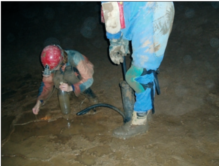
Figure 74: Apparatus for aspirating water in pools. After aspiration, the water is filtered through a net or filtering bottle (Fig. 73) in order to recover the epikarst fauna (Photo: Daniel W. Fong).
