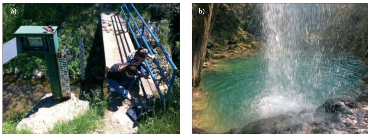
Figure 81: Butori watercourse: a) limnigraphic station with part of the team the Civil Engineering Faculty of Rijeka (Photo: Igor Ružić), b) Butori waterfall in the area of the ponor (Photo: Josip Rubinić).
