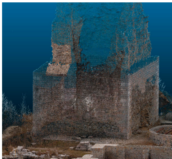
Fig. 13.3: 3D scan of the Smednik Castle ruins in 2007, close-up view of the point-cloud of the tower, entrance above the current ground. Due to the low point cloud density measuring the height of the entrance above the ground level was a demanding task to be performed merely with the use of the point cloud data.
