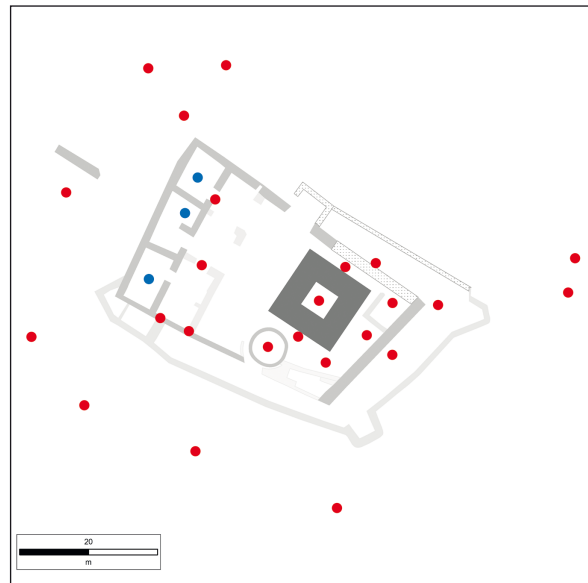
Fig. 13.6: The locations of scanning positions in 2007 (red) and the “missing” positions (blue) that should have been used in addition.
