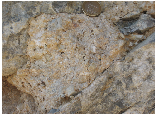
Fig. 9.4: The mortar used in the construction of the tower was made from dolomite chippings, sand and lime. Chippings measure up to 2 cm. View 2.
