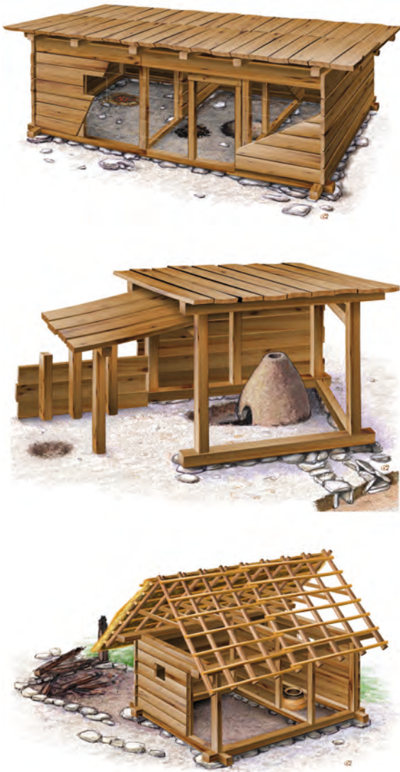
Sl. 5: Rekonstrukcije hiš 15A, 23 in 16 (risba: I. Rehar). Fig. 5: Reconstruction of Houses 15A, 23 and 16 (drawing: I. Rehar).
