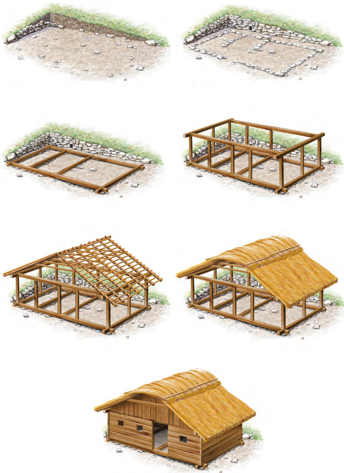
Sl. 8: Rekonstrukcija gradnje hiše 8 (risba: I. Rehar). Fig. 8: Reconstruction of House 8 construction (drawing: I. Rehar).
