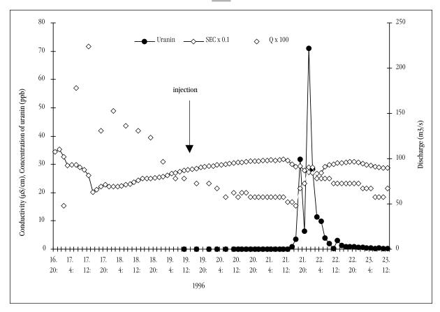
*Fig. 1.8.6. Stream flow at Dakenyan: comparison of discharge, SEC and uranin appearance in July 1996.*
