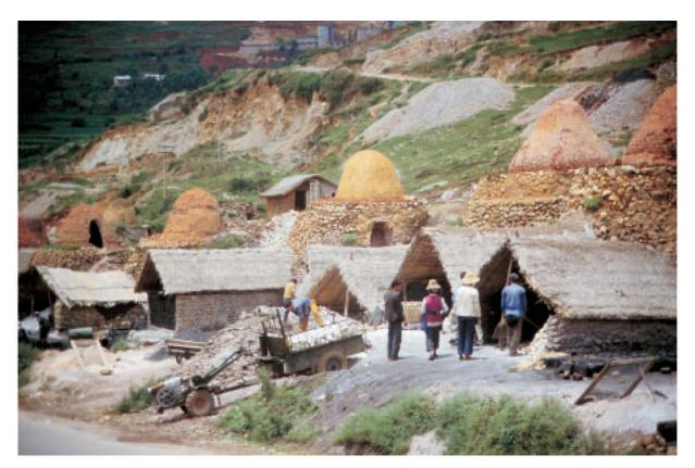
Fig. 2.10.16. Traditional form of lime-kiln. Coke is used for burning (Photo A. Mihevc).
