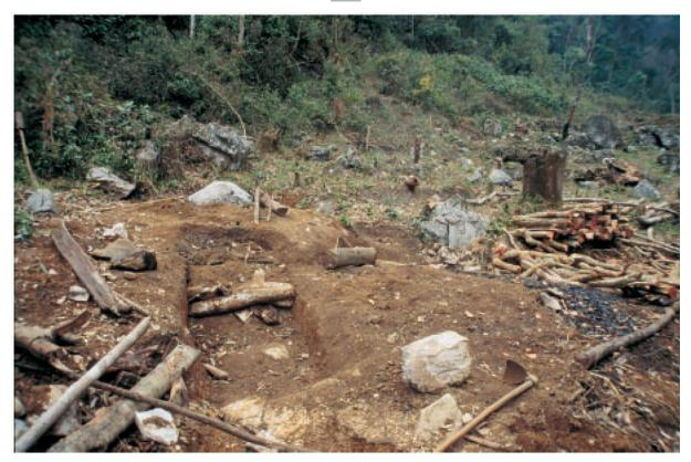
*Fig. 2.10.14. Charcoal is produced in underground stoves. The furnaces are located where there is enough wood and where the terrain is less rocky (Photo A. Mihevc).*
