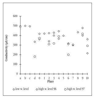
Fig. 1.8.4. SEC of water at measurement points during very high and during low water levels.
