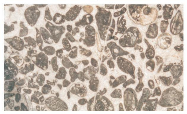
Figure 2.6.7: Weel sorted bioclastic peloidal grainstone. Bioclasts (fusulinids, gastropods, and individual crinoidal plates) are partly rounded, micritized, and some are even coated.
