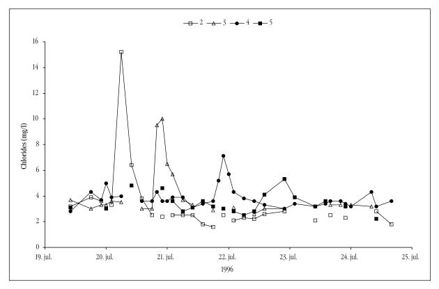
Fig. 1.9.14. Breakthrough curves of NaCl at the Points 2, 3, 4 and 5.
