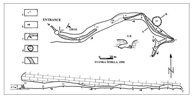
Fig. 1.2.11. Map of cave Guan Yin Dong (ground plan, longitudinal and cross sections); a-point of cave measurements, b-direction of water flow, c-strike and dip of bedding planes, d-collapse doline, e-water flow.
