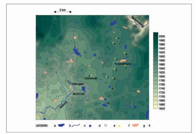
Fig. 1.7.1. Hydrological map of the Tianshengan area (a-lake, b-surface stream, c-bigger spring, d-smaller spring, e-shaft with underground water flow, f-village, g-mark of the hydrological object - see also chapter 1.9.).
