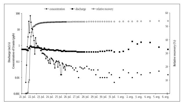
Fig. 1.9.13. Discharge, breakthrough curve of Uranine and relative recovery of Uranin at Dakenyan Point 4.
