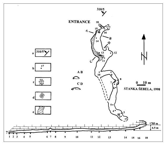
*Fig. 1.2.10. Map of cave Xin Shi Dong (ground plan, longitudinal and cross sections); a-strike and dip of bedding planes, b-point of cave measurements, c-collapse blocks, d-flowstone, e-lake.*
