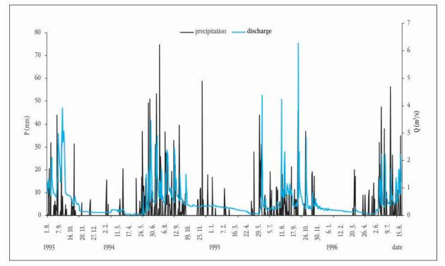
Fig. 1.7.8. Diagram of daily precipitation and discharge for the period of 1.8.1993 to 21.8.1996.
