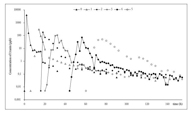
Fig. 1.9.12. Breakthrough curves of Uranin at the points 0, 1, 2, 3, 4, and 5.
