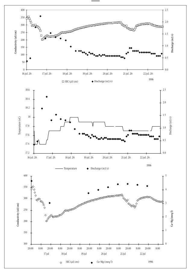
Fig. 1.8.5. Accurate recording of discharge, temperature and SEC with occasional analyses of total hardness of groundwater flow at Dakenyan (4) in water pulses in July 1996.
