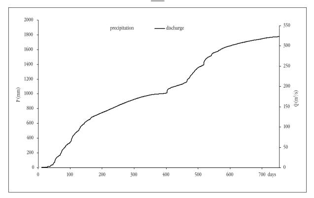
*Fig. 1.7.10. Cumulative curves of precipitation and discharge for the period of two hydrological years.*
