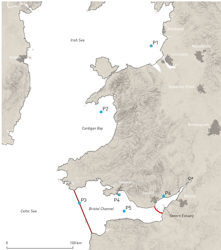
Figure 37: Locations of observation points for the analysis of water elevation changes due to the barrage operation. SE model computational domain boundary is shown in dark red, the barrage in light red.
