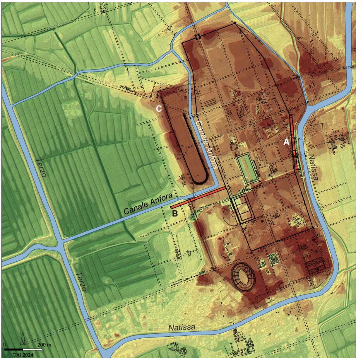
Fig. 5: Terrain model of Aquileia based on Lidar data with the course of rivers and canals, the street grid and selected features. A – Harbour on the Natissona; B – Harbour on the Canale Anfora; C – Early Christian basilica (ÖAW/ÖAI, H. Sedlmayer).
