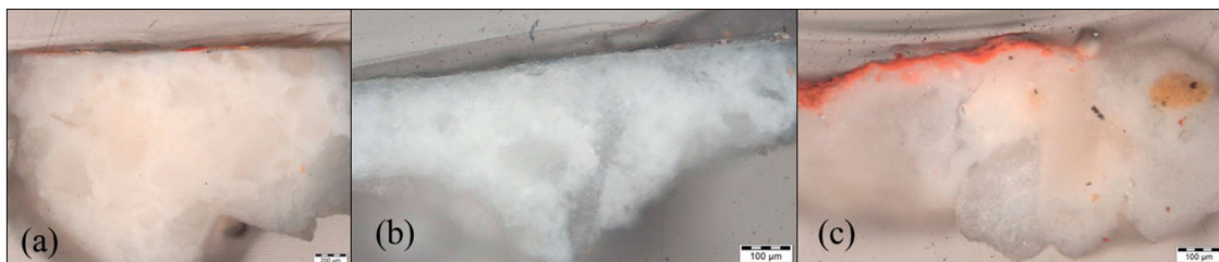
3. Microphotographs of plaster samples and colour layers using optical microscopy in reflected light from the following locations: (a) St Thomas's church in Velike Poljane, (b) St Thomas's church in Gorenja Straža, and (c) St Michael's church in Biljana. All plasters are white and consist of lime and crushed calcite (© IPCHS, RC, Scientific department).
