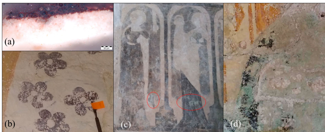
6. Colour darkening due to pigment degradation, observed on the sample microphotograph (a) and in situ (b, c, d) in the following locations: (a, b) Pb pigment (?), St Peter's church in Ribičje, (c) Pb and/or Cu pigments, St James's church in Ormož (central nave), and (d) malachite, St Nicholas's church in Žužemberk (St. Erasmus) ((a) © IPCHS, RC, Scientific department; (b-d) photos: Anabelle Križnar).
