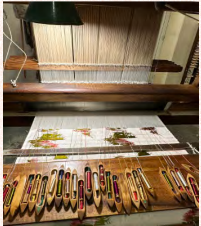
Shuttles of silk threads in colors allow to create a complex pattern. Foto: Verena Gruber.
