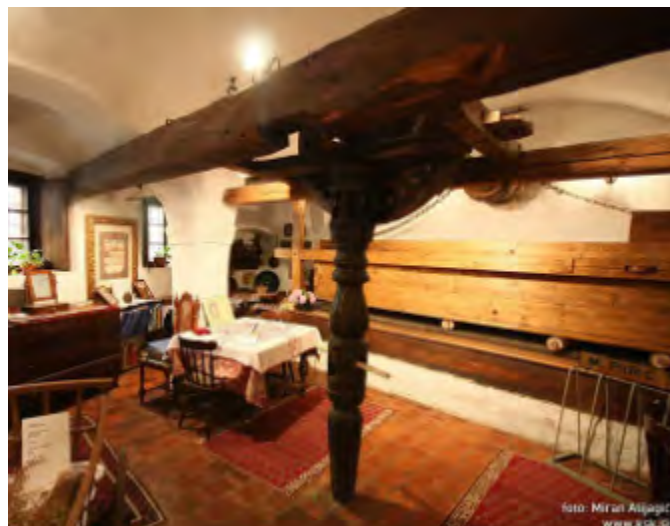
"Monga", device for ironing fabrics in Pirc dye house in Kranj. Source: KSK Foto
