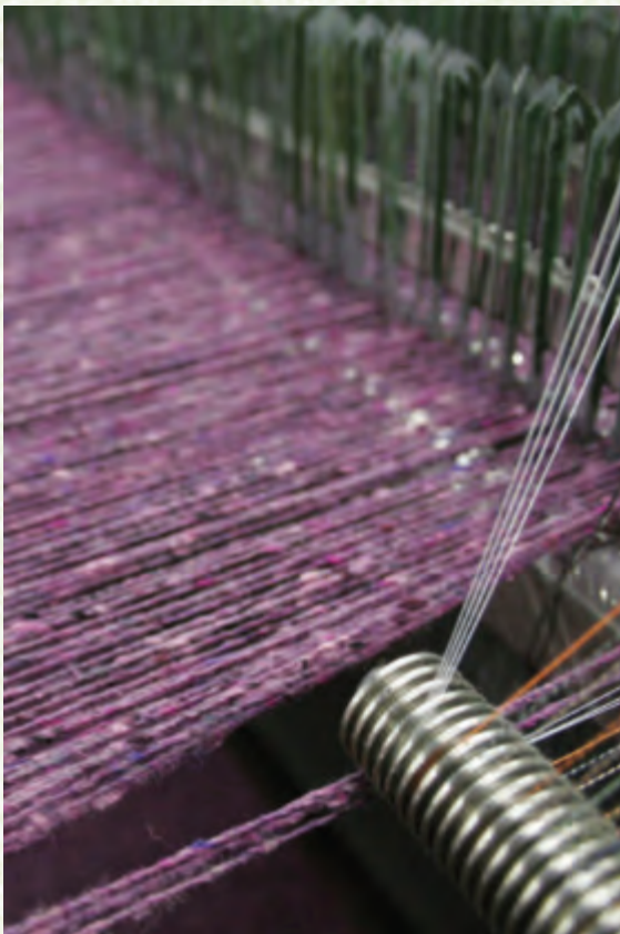
Lanificio Paoletti, the warp yarns of wool on the loom. Source: Lanificio Paoletti.
