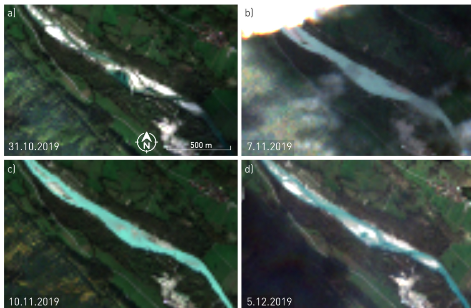
Figure 49: Sentinel-2 true colour images showing the removal of gravel from the Soča river at the Dolje study area and the subsequent formation of new gravel bars. The extent of gravel bars under observation is shown on Figure 47. Data source: Modified Copernicus Sentinel data, 2021.
