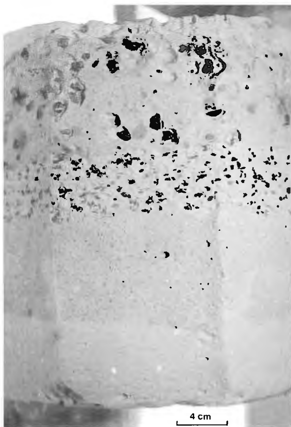
2.3.16 Scallops on bedded block of plaster
