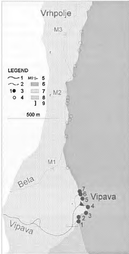
Figure 6: Permanent and intermittent Vipava springs (1. The Vipava River, 2. Temporary surface stream, 3. Permanent Vipava springs 1-7, 4. Intermittent spring, 5. Point of discharge measurement, 6. Karst aquifer, 7. Alluvial deposits, 8. Flysch, 9. Gauging station)
