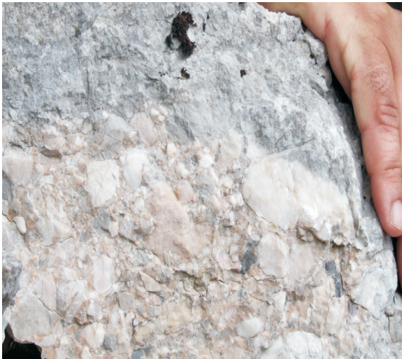
Fig. 12: The Jelar Breccia is a massive, thick-bedded carbonate rock, comprised predominantly of angular, poorly sorted debris; North Velebit (photo: N. Zupan Hajna).
