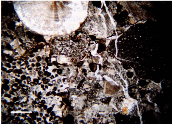
Fig. 3.65 Member 4 of the Travnik Formation: carbonate breccia with lithoclasts of the Members 1,2,3 of the Travnik Formation, belemnites and peloids (section MA1). Scale bar is 1 mm long.
