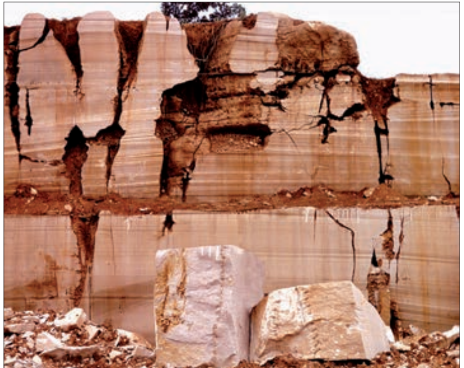
Figure 3: Parts of faces 1 (top) and 2 (bottom) used in the data analysis. Cutters are narrower and more closely spaced than in Figure 2. In face 1 (top), the measured sample includes the six main cutters but excludes the thin fissure at right. Width of view is 9 m. In face 2 (bottom), the sample includes only the two largest cutters. The narrow fissures are simply sawed grooves.
