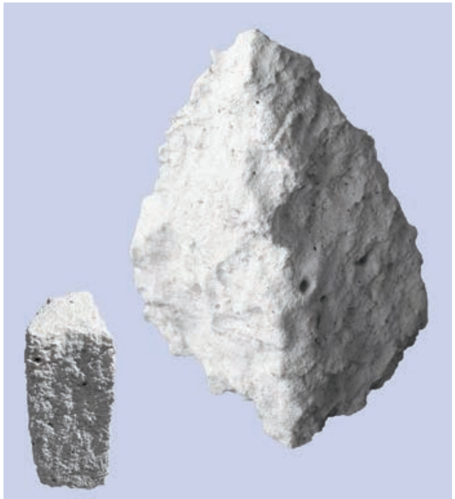
Figure 4: Development of gypsum subsoil pillar; left: early stage, right: final stage of experiment.
