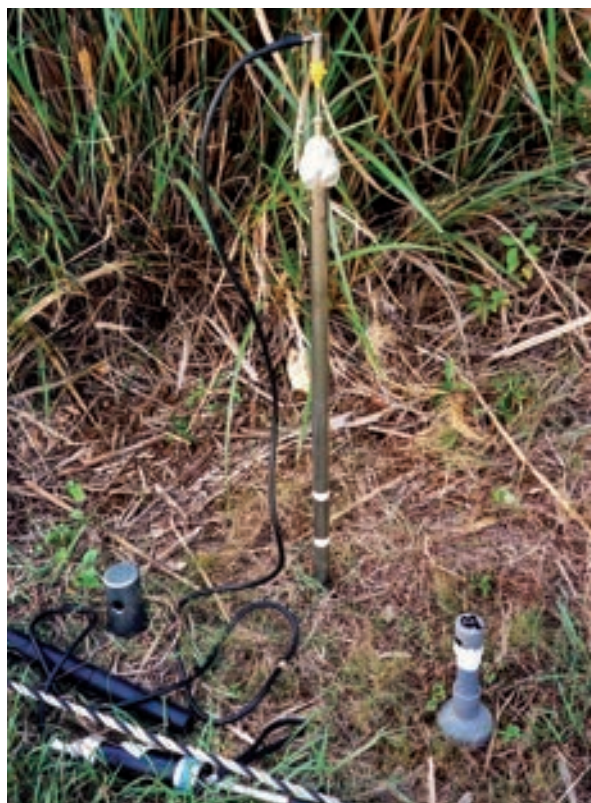
Figure 6: The CO 2 measurement in Minamidaito island (upper Dräger method, lower Gastec method).
