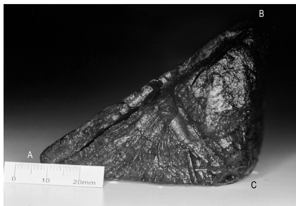
Sl. 8.31: Zagozda B2. Pogled v smeri osi. Foto: M. Pflaum. Fig. 8.31: Wedge B2. View in direction of axle. Photo: M. Pflaum.
