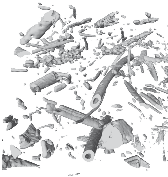
Sl. 17.1.2: Sistem por v agregatu iz frakcije 3–10 mm. Mikro TC posnetek je bil narejen na Zavodu za gradbeništvo v Ljubljani. Fig. 17.1.2: System of pores in the aggregate from the 3–10 mm fraction. The micro TC picture was made at the Slovenian National Building and Civil Engineering Institute in Ljubljana.
