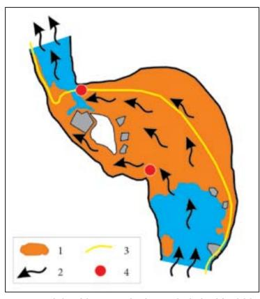
Fig. 2: Ground plan of the rimstone dam between the third and fourth lakes (1 – rimstone dam, 2 – watercourse, 3 – tourist path, 4 – micrometric points).
