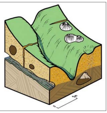
Fig. 6: Karst in breccia in contact with flysch.
