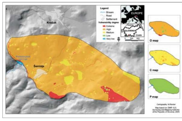
Fig. 3: Example of groundwater resource (aiming to protect the whole groundwater body) vulnerability map according to the Slovene Approach (Ravbar 2007).
