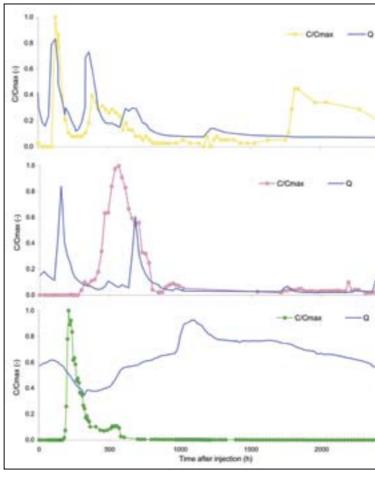
Fig. 4: Discharges and concentrations of tracer (standardised with regard to the maximum measured value) in the most important springs from the time of injection of the tracer.
