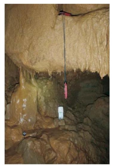
Fig. 1: Measurement of selected ecological characteristics in Piskovica cave habitat with set of mobile instruments (photo: R. Ozimec).
