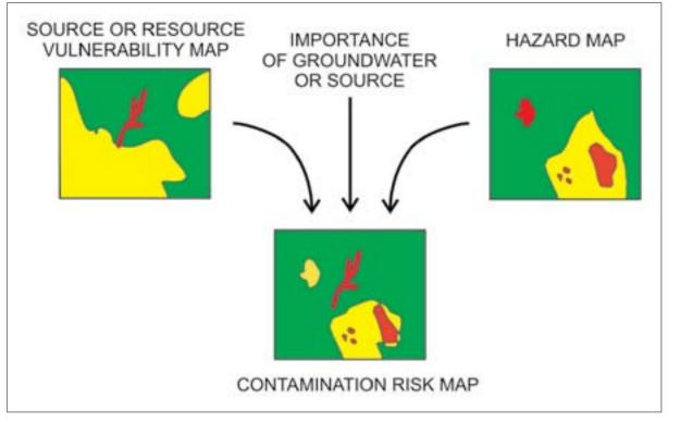
Fig. 2: Groundwater vulnerability and risk to contamination assessment scheme.
