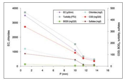
Fig. 2: Progress of measured parameters of oil collector inflow (EC, COD and BOD.) following a precipitation event on 24 March 1993 depending on the quantity of precipitation.
