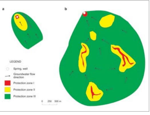
Fig. 1: Arrangement of source protection zones a) based on transit time or distance criteria, typically in granular aquifers and b) considering special characteristics of water flow in karst aquifers.
