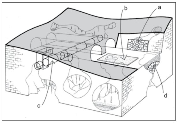
Fig. 1: Cave preservation, a - in road cuts, the caves are hidden behind rocky scarps, b - the caves lying below the road with narrowmouths and, if their rim is not damaged too much by blasting, are covered by concrete lids, c - in the side of the tunnel pipe there is a special door which leads to the caves. Below, road caves are connected with large concrete pipes, d - karst openings (bottom of dolines, tops of shafts) are often reinforced by arches of large rocks which concrete poured on top.
