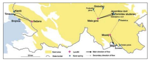
Fig. 1: Directions of flow from landfills on karst in S Slovenia as known by tracer tests.
